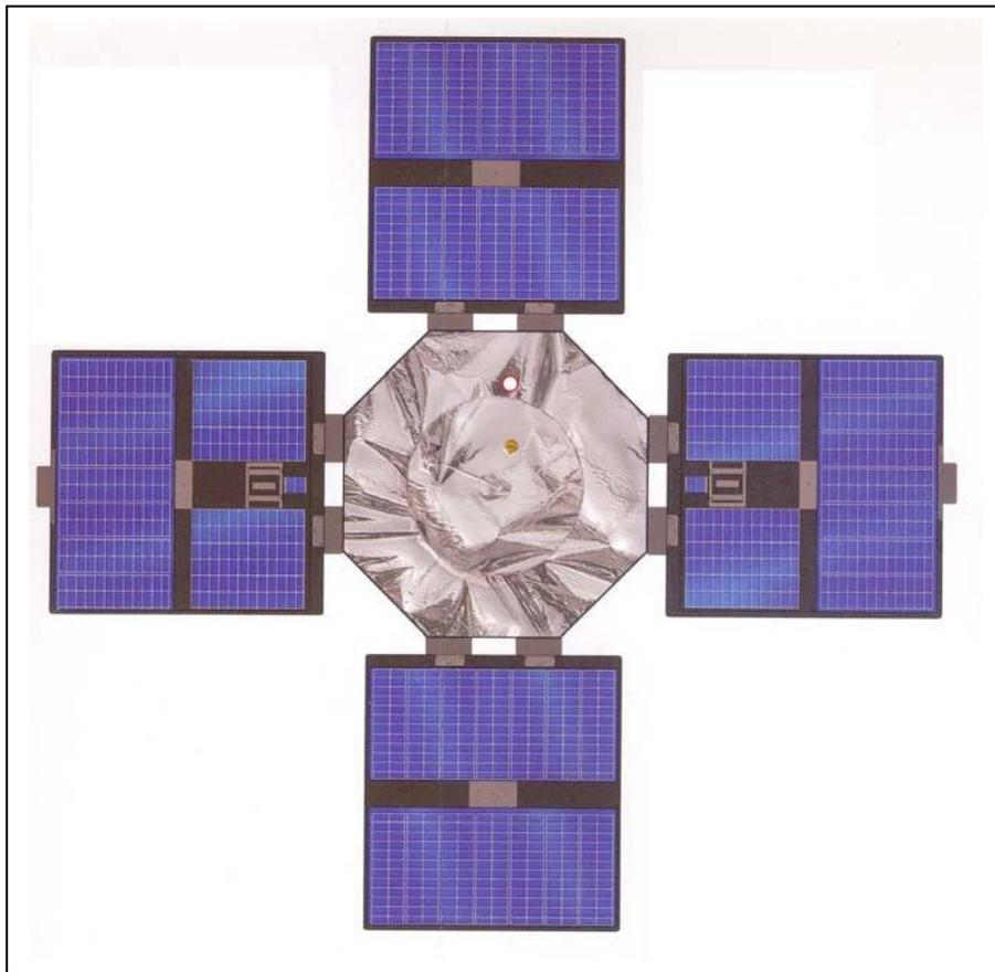
NASA's twin Van Allen Probes were launched in 2012. The figure above shows the octagonal spacecraft body and the location of the surrounding four solar panel 'wings' that provide power to the spacecraft instruments. The small blue rectangles within each of the four solar panels show the location of the solar cells used to power the satellite. As the spacecraft orbits Earth, the four solar panels continuously face the sun to provide constant power.
