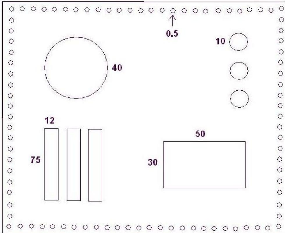
This is a diagram of a panel from a spacecraft showing all of the openings. All units are in centimeters. The panel is 190 centimeters wide and 150 centimeters tall. The diameters of each circular opening is also given. The small holes around the circumference are for the screws that fasten the panels together.
