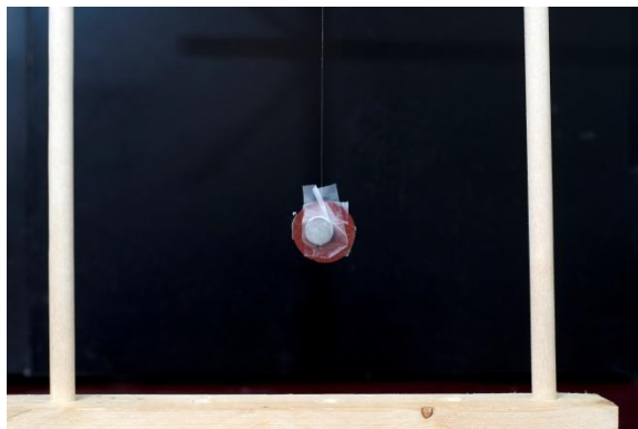
Figure 4: Rare-earth button magnet shown adhered to the back of a small mirror and suspended using a length of fishing line.
