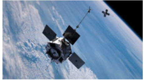
Figure 1. The identical Van Allen Probes follow similar orbits that take them through both the inner and outer radiation belts. Image courtesy: JHU/APL
