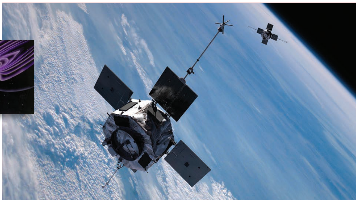
Image credit: JHU/APL. The identical Van Allen Probes will follow similar orbits that will take them through both the inner and outer radiation belts. The highly elliptical orbits range from a minimum altitude of approximately 373 miles (600 kilometers) to a maximum altitude of approximately 23,000 miles (37,000 kilometers).
